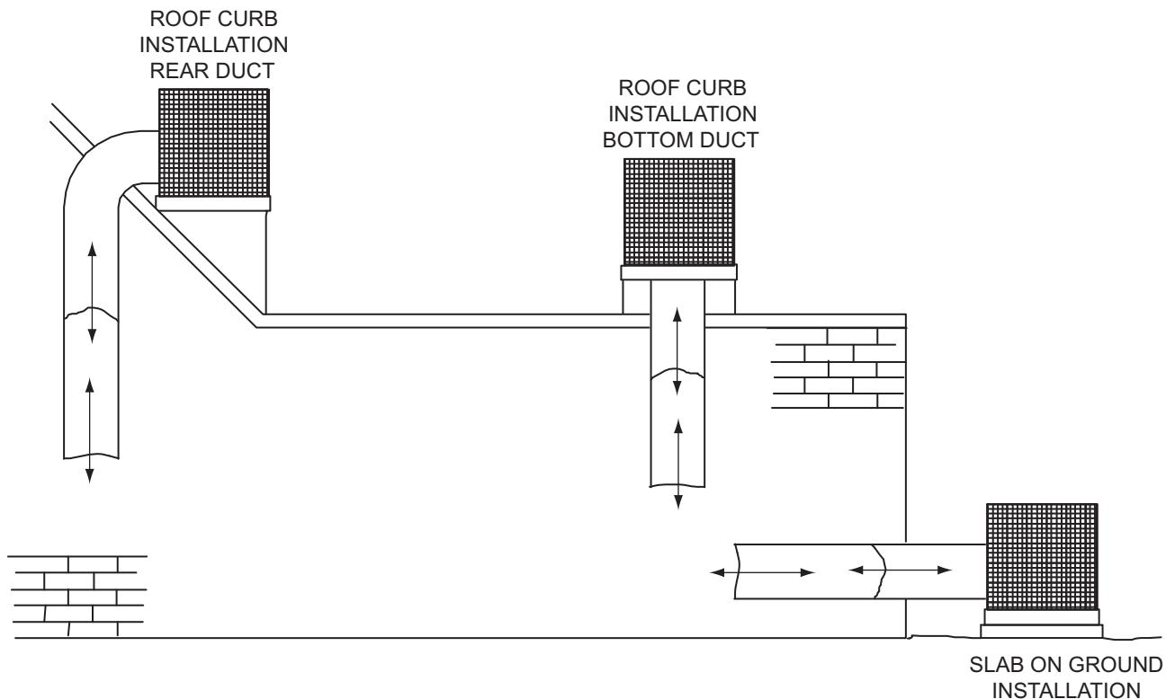
**Unit Typical Slab on Ground Installation**
